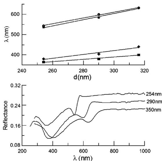
FIG. 4. Scaling of the reflectance spectrum of nanocorrugated films with the diameter of the particles of the colloidal crystal. Upper graph is the positions of lw and sw reflectance minima for the samples with different diameters (Co thickness is 30 nm) for the incident angle 20°: Circles and squares—s-polarization, stars and crosses—p-polarization. The bottom graph is the reflectance spectra for s-polarized light with the angle of incidence 20°.
