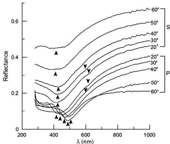
FIG. 3. Measured optical reflectance spectra of 60 nm thick nanocorrugated Co film (particle size of initial PMMA colloidal crystal is 290 nm) for s- and p-polarization of the incident light and for different incident angles. Up arrows indicate minima due to localized dipole mode; down arrows indicate remnant minima due to propagative surface plasmon mode.
