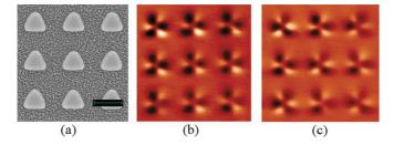
FIG. 1. (Color online) (a) Scanning electron microscope (SEM) image of the lattice of the cobalt triangles, the scale bar length is 1  $\mu$ m. (b) MFM image of the remanent states after magnetizing along the base of the triangles. All magnetic vortices demonstrate the same direction of the vorticity. (c) MFM image of the remanent states after magnetizing along the height of the triangles. The vortices with both CW and CCW vortices are presented.
